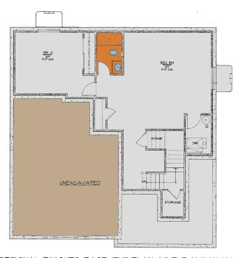
OPTIONAL FINISHED BASEMENT PLAN AT ELEVATION 'A'
